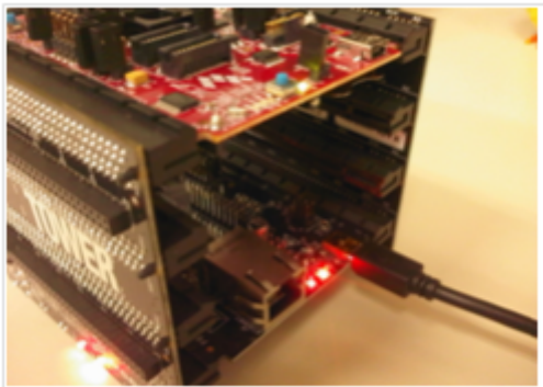
Figure 30. Connecting the USB cable
